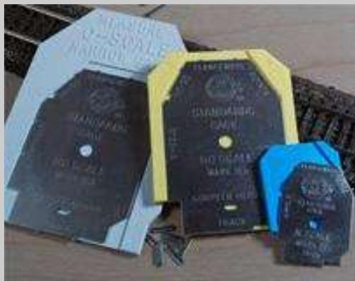
You may not realize that the NMRA sells clearance gauges in On30, HO, and N scales. When you're running On30 or post-1983 N- or HO-scale equipment, you need more than the standard, metal NMRA gauge.
